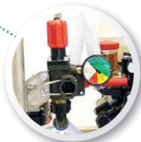
WATER PUMP CONTROLLER
